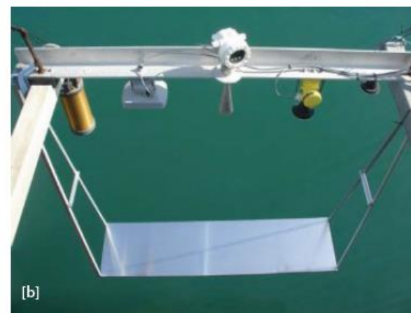
Figures 1 [b], [c]. The same frame and gauges with a metal target (stirrup) suspended beneath them.
