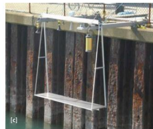
Figures 1 [b], [c]. The same frame and gauges with a metal target (stirrup) suspended beneath them.
