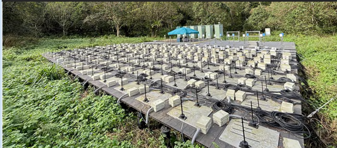
Taiwan's BURSTT array uses 256 radio antennas to monitor half the sky at once. KAI-YANG LIN/ASIAA
