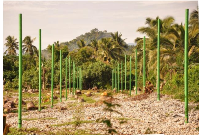
Receiving Array 8 MHz range 250 km
