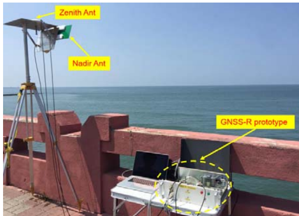
Fig. 6 Ground test with GNSS-R prototype
