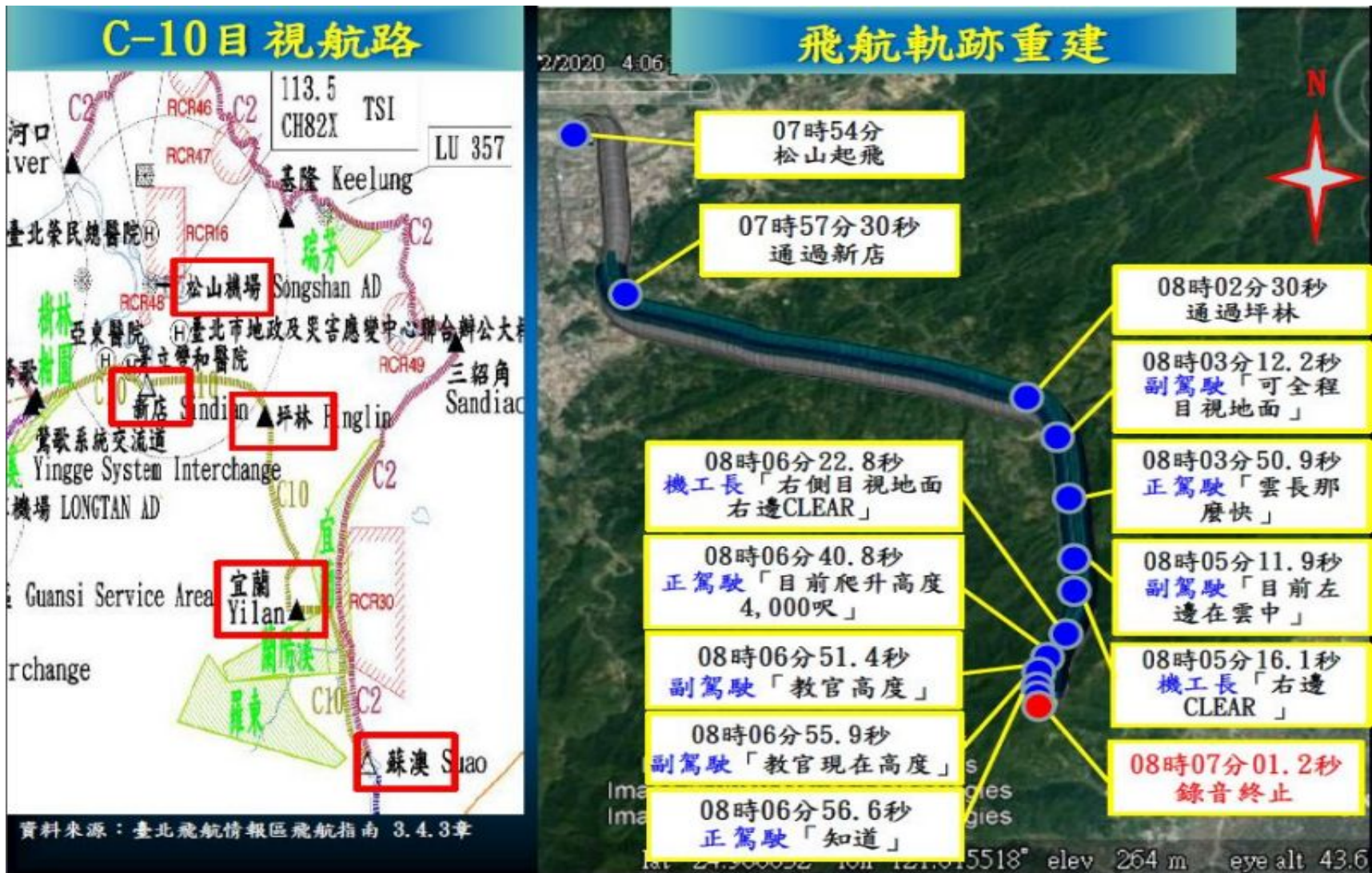
Fig. 13. (a) The C-10 visual flight route map. (b) The reconstruction of flight trajectory for ROCAF UH-60M helicopter on 2 January 2020, including time(TST), and dialogue remarks in the cockpit. (Referred from the ROC MND Preliminary Investigation Report of the UH-60M Incident on 15 February 2020)
