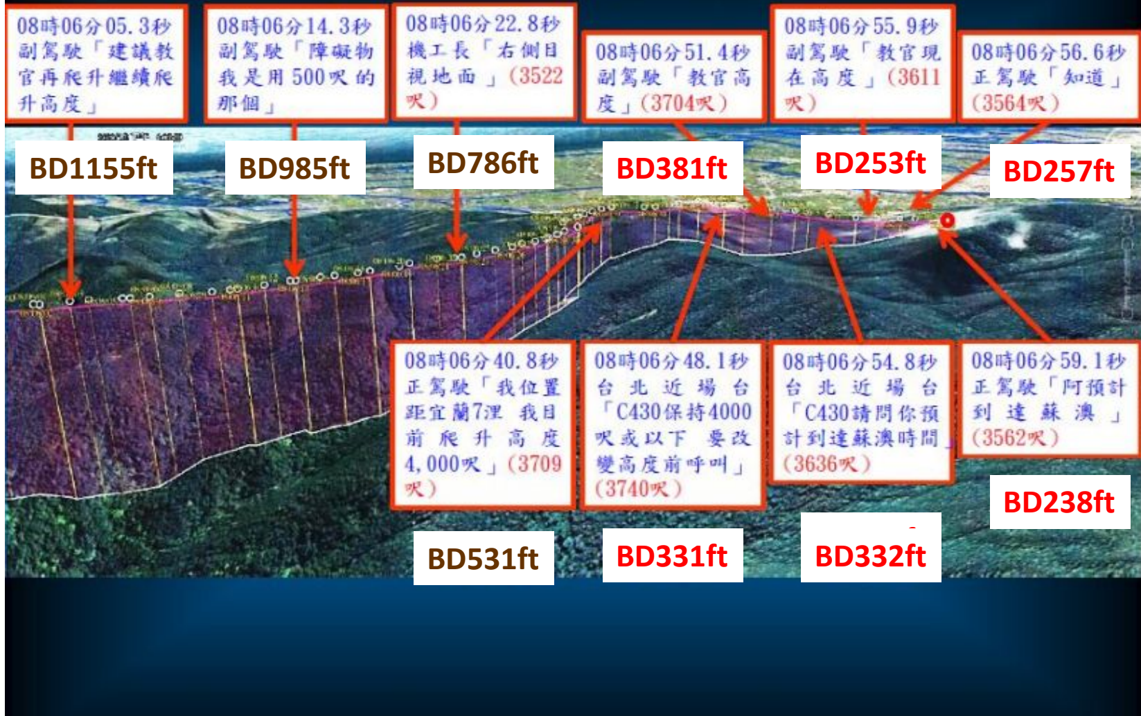
Fig. 15. The overlay of flight trajectory and topography during the last minute before ROCAF UH-60M helicopter accident on 2 January 2020, including time(TST), plane altitude(ft), and dialogue remarks in the cockpit. (Referred from the ROC MND Preliminary Investigation Report of the UH-60M Incident on 15 February 2020)
