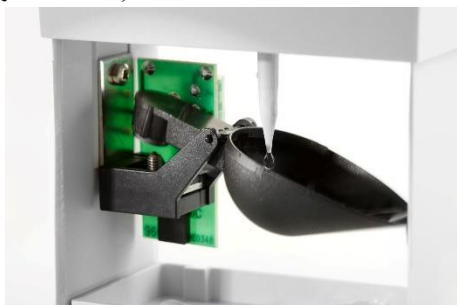
圖 2 Tipping spoon (PRONAMIN, Rain-O-Matic)
