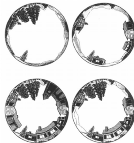
Figure 2. Diagrams of gauge sites with four different degrees of protection against wind by trees and houses, as taken using a camera with a fish-eye lens through the gauge orifice. Clockwise: open site, partly open site, partly protected site, and protected site
