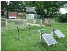
Fig. 1. The instruments deployed in the NTU. From near to far: two Parsivel, two rain gauges (0.5 mm and 0.2 mm resolution), one JWD, and the VPR.
